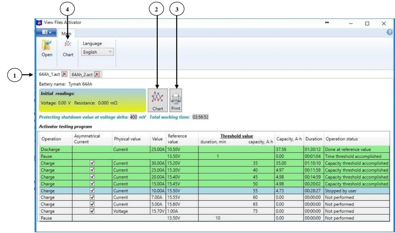
4) "Chart" button. In case if there is only one activator file is loaded, it works similar to "Chart" button described before. If there are more than one loaded activator files, all charts will be shown. Line color coding will be shown to the right of the charts.
